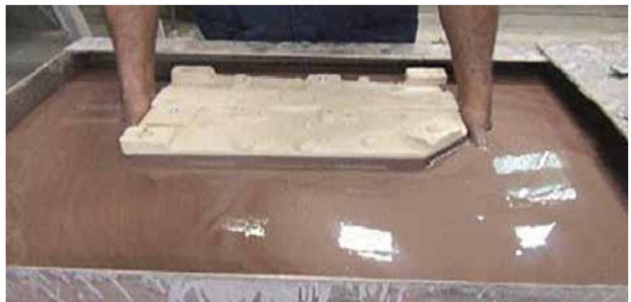
Figure11: Assembly tilting for paint dropping to avoid run down and droplets
