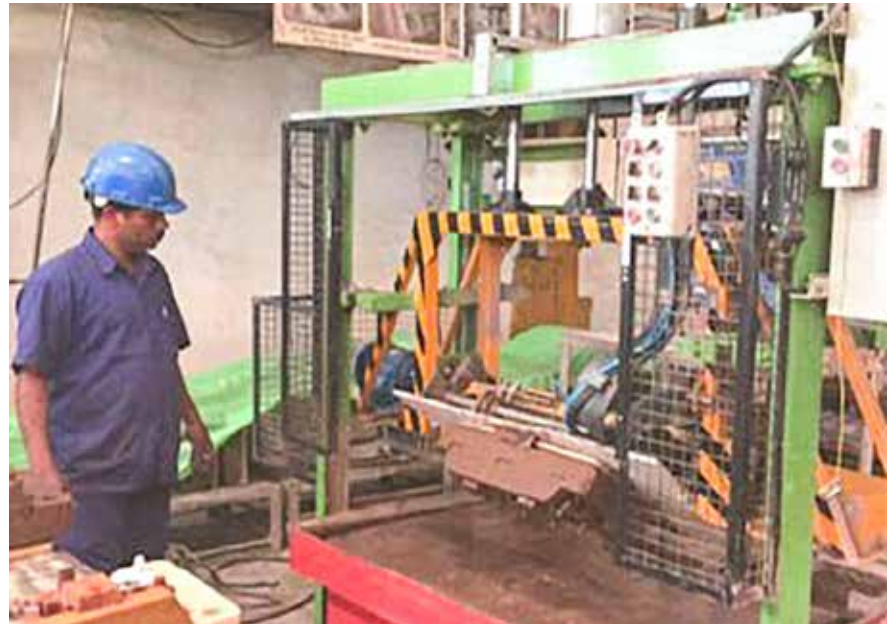
Figure14: Core assembly dipping with predetermined cycle
