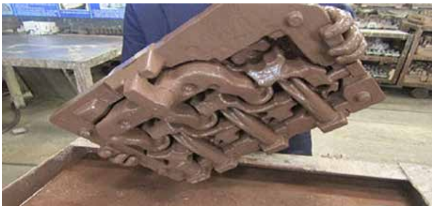
Figure11: Assembly tilting for paint dropping to avoid run down and droplets
