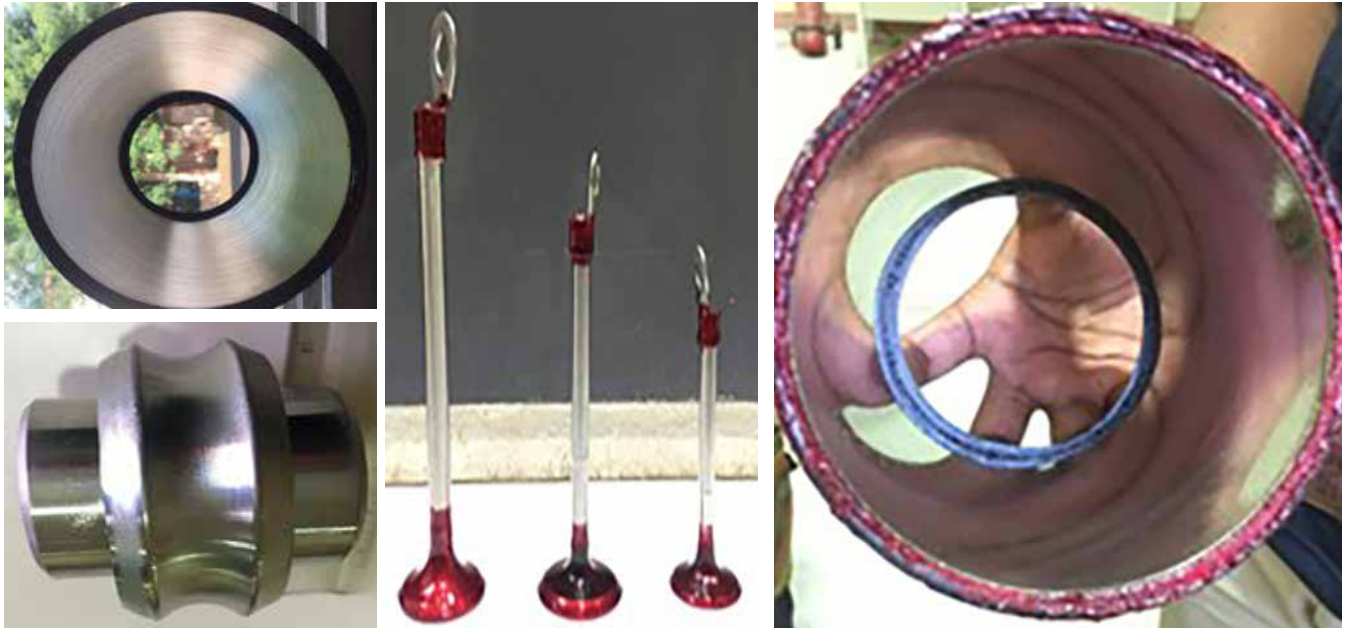
Figure9: Various industrial components coated with PED technology at ARCI
