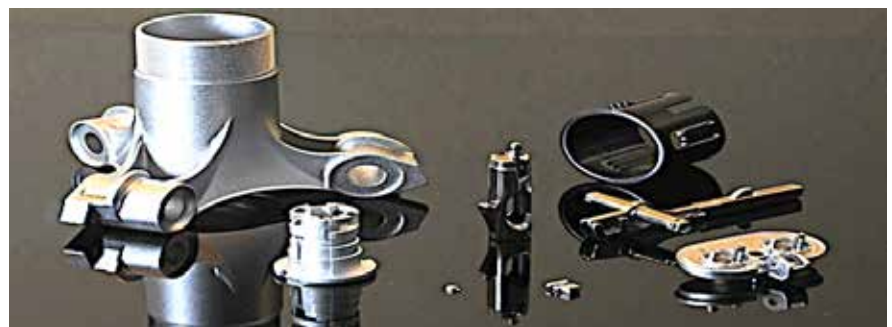
Figure7: Part samples produced by PIM method
