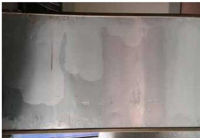
Aluminium foam core 2014 Al-alloy (0.5 mm thickness) faced sandwich panels (size 1m x 2m x 0.025 m) (areal density: 3.5 kg/m 2 )
