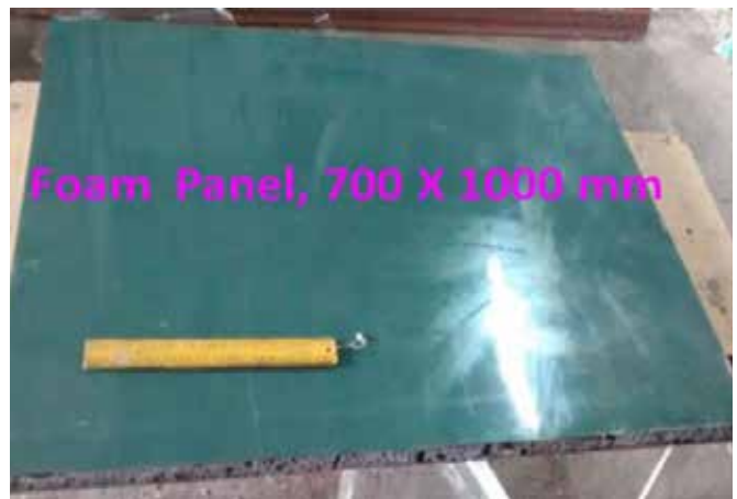
FRP faced Al-foam core sandwich panel, 30 mm thickness (areal density: 7.0 kg/m 2 )
