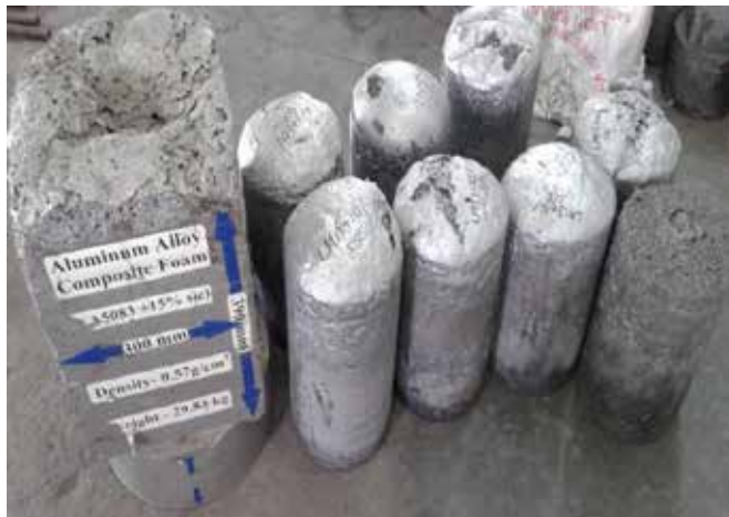
Foam billets made at 80 percent reproducibility, large size foam billet preparation demonstrated
