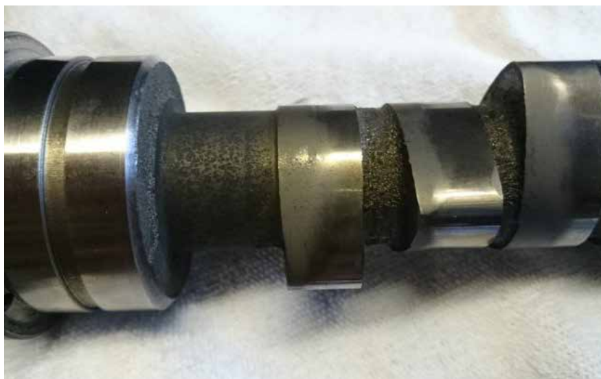
Figure10: Heavy pitting observed
