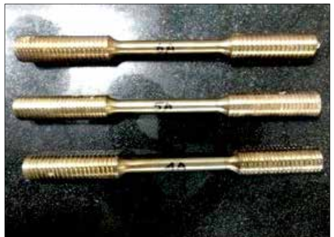
Figure9: Tensile sample with heat tint mark
