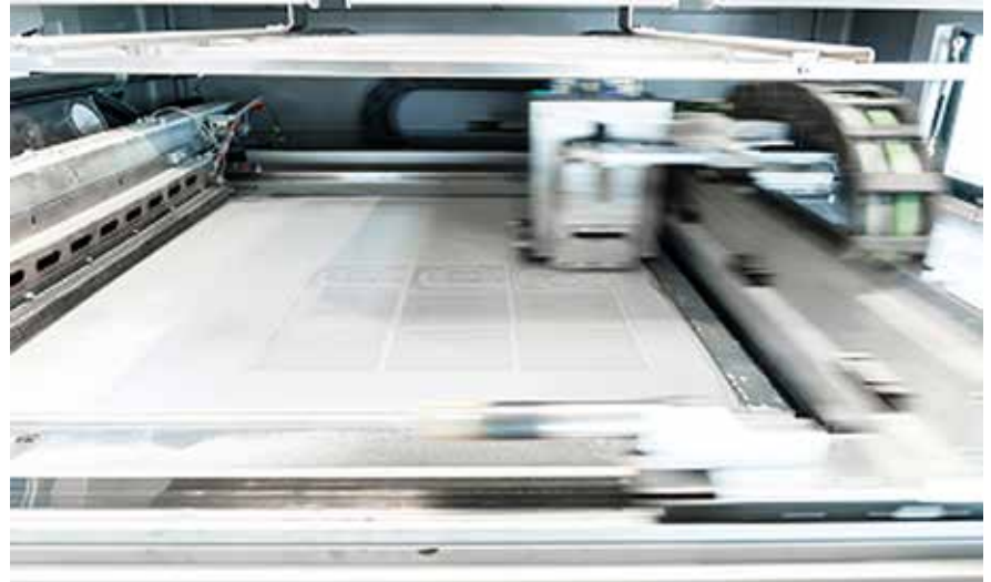
Figure10: Print-head and building platform in VX I 000
