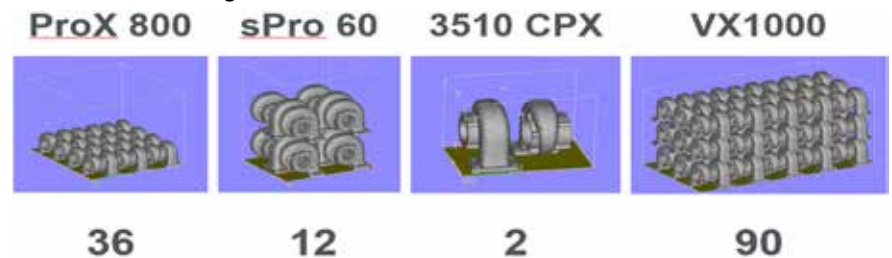
Figure9: Direct nesting comparison of additive technologies for investment casting
