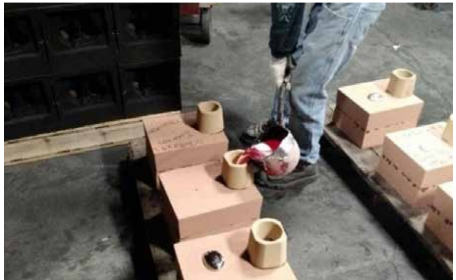
Figure5: Pouring raw castings from hybrid composite material
